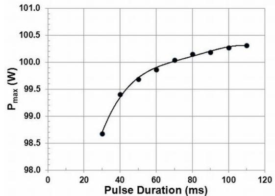
**Figure 7:** Dependence of measured maximum output power ( $P_{max}$ ) for a commercial thin-film CIGS module on the duration of the light pulse used to test the module. For this module, it is apparent that an underestimate of possible maximum output power of nearly 2% can occur if one were to utilize a pulsed simulator of insufficient pulse duration.
