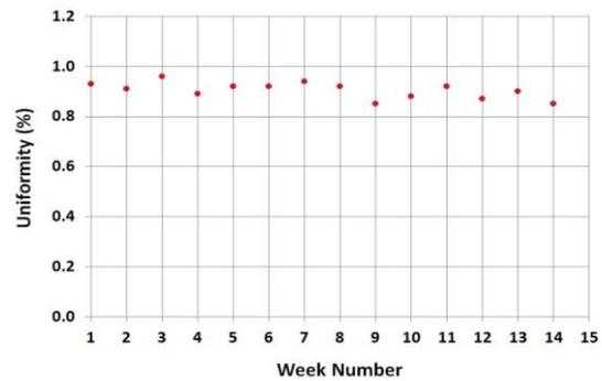
**Figure 4:** Temporal stability of spatial uniformity of a 5600SLP Blue simulator over a 14-week period. No adjustments to the uniformity hardware or to the lamp balance were made during this period.
