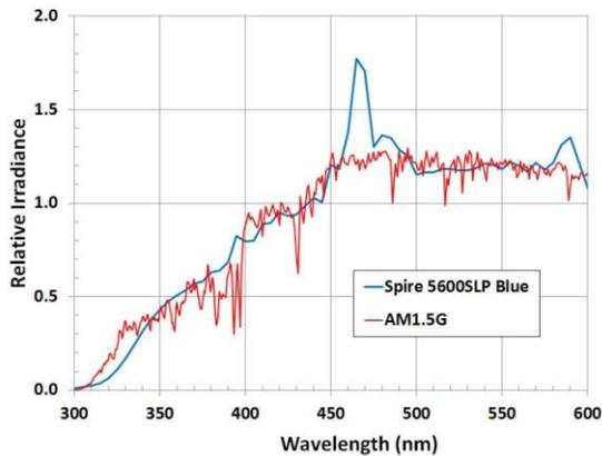
**Figure 2:** Comparison from 300 to 600 nm of the 5600SLP Blue spectrum to AM1.5G showing the excellent match over this wavelength region.
