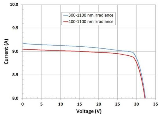
**Figure 5:** 1-sun IV curves for a selective emitter (SE) crystalline Si module tested under standard 400-1100 nm illumination and UV-enhanced (300-1100 nm) illumination.
