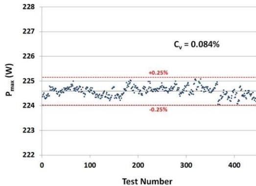
**Figure 9:** Long term  $P_{\max}$  measurement repeatability of the 5600SLP Blue. Here a total of over 450 measurements was conducted during a 6-month period. The  $C_v$  for these tests was approximately 0.084%. Reference lines indicating  $\pm 0.25\%$  about the mean are shown.
