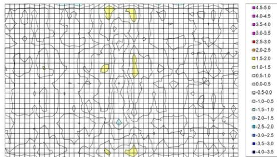
**Figure 3:** High resolution (570 pixels/m<sup>2</sup>) uniformity map over the 1.37 m x 2.00 m output test plane of a 5600SLP Blue. White areas correspond to less than  $\pm 1\%$  irradiance variation at high resolution from the mean, while the yellow and blue areas correspond up to  $\pm 1.5\%$  deviation, respectively. The corresponding standard resolution 25 pixel/m<sup>2</sup> uniformity defined by the IEC standard is  $\pm 0.72\%$ .
