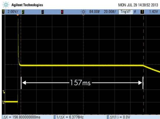
**Figure 6:** Oscilloscope trace of the optical pulse intensity of the 5600SLP Blue simulator at an irradiance level of 1000 W/m<sup>2</sup>. The flat portion of the pulse has a duration of nearly 157 ms.
