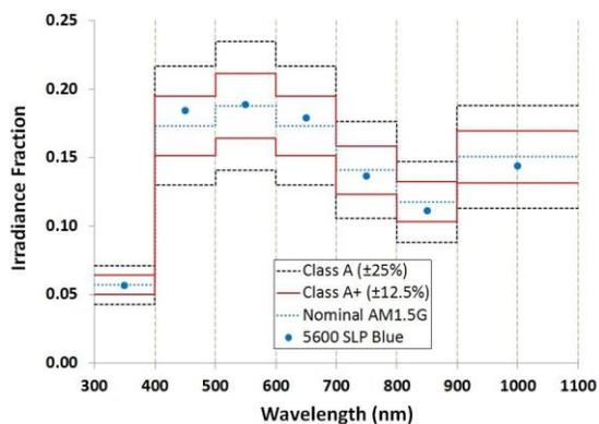
**Figure 1:** Spectrum by wavelength bin from 300 to 1100 nm for the Spire 5600SLP Blue simulator. The red lines (Class A+) indicate  $\pm 12.5\%$  deviation from AM1.5G.
