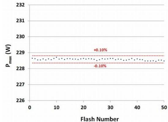
**Figure 8:** Short term  $P_{max}$  measurement repeatability of the 5600SLP Blue. A total of 50 flashes was made over a ~30 minute period. Reference lines indicating  $\pm 0.10\%$  about the mean are shown.
